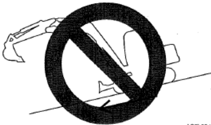
Steep slope when the attachment is lifted
