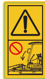
21. Keep the boom and bulldozer separate. When lowering the boom, be careful not to let the boom come into contact with the bulldozer blade.
